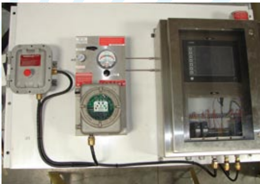
PURGED PLC AND SCREEN CONTROL PANEL FOR OFFSHORE RIG
